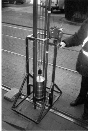
Figure 6: Falling weight device for an impact excitation
